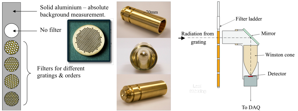
Figure 1.21: The optical parts of the E-203 experiment: (from left to right) the filters, the optical concentrators (winston cones) and the optical assembly (image taken from [43]).
