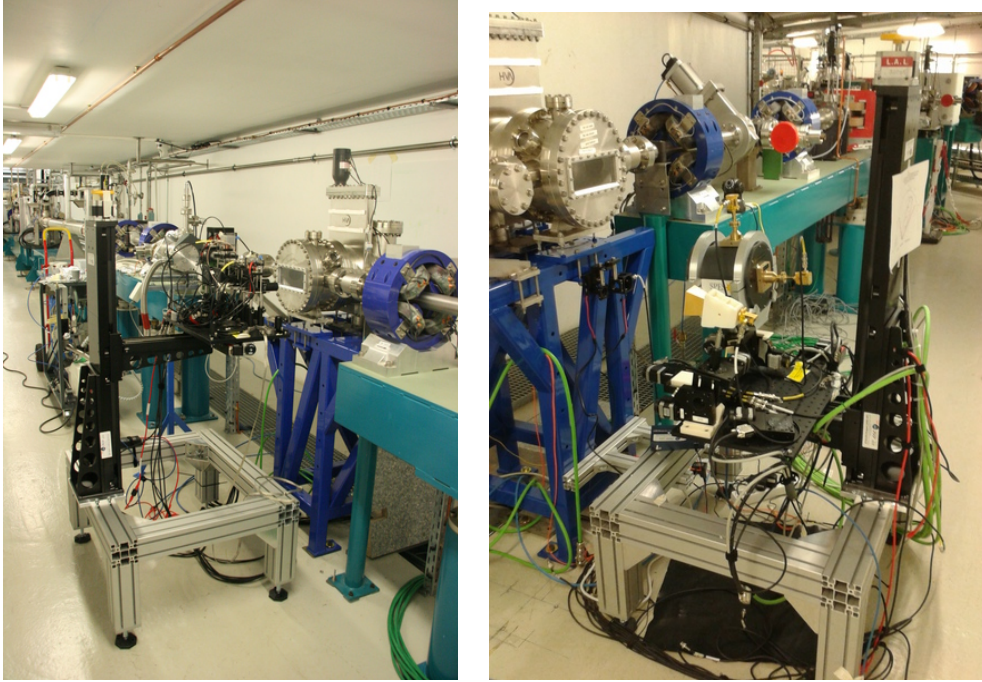
Figure 8.25: The experimental setup of SPESO at the end of the SOLEIL Linac: left, as it was in 2015 (image taken from [146]) and right with the polarizer installed in 2016 (image taken from [147]). On both images the electrons travels from left to right.
