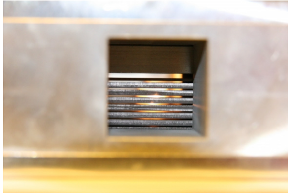
Figure 7.4: Picture of the pepper-pot used at the BTF as shown in [75].
