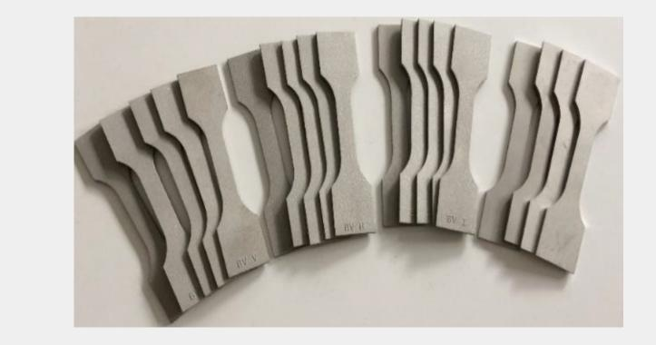
Several samples printed using additive manufacturing with different machine settings or sample orientation. Source: Stéphane Jenzer (LAL, Orsay).
