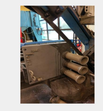
Beam-pipes after they have been produced by additive manufacturing and before they were removed from the support IPAC'17 (source: *WEPVA043*).
