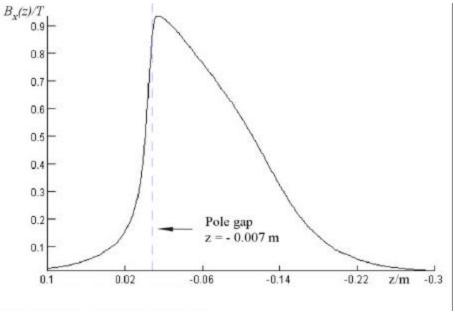
Figure 2 Cross section of the field in the z-direction for x = 0 and y = 0.
