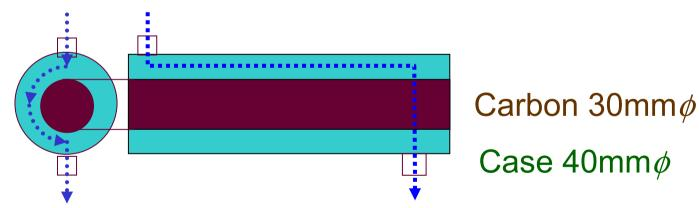
measure flow rate and temperature difference.
