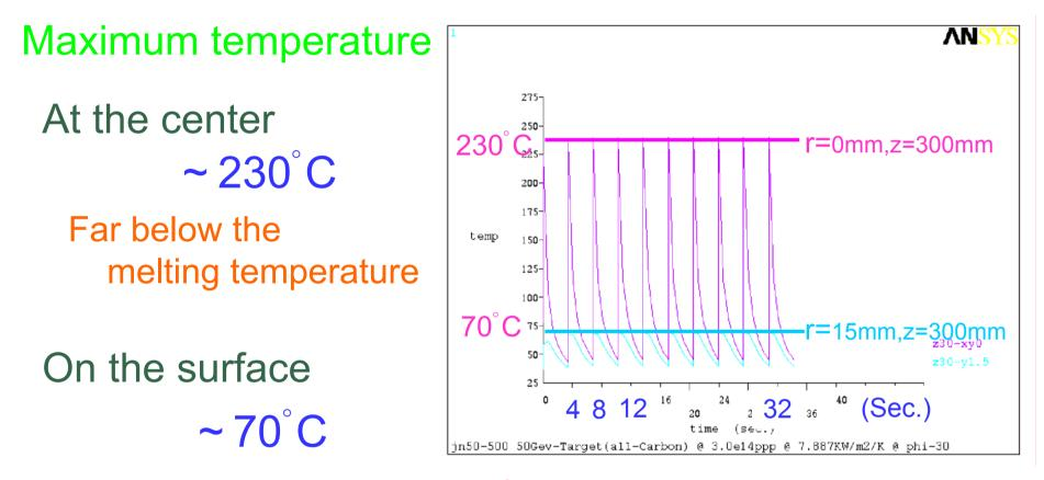
This should be lower than 100°C for water cooling.
