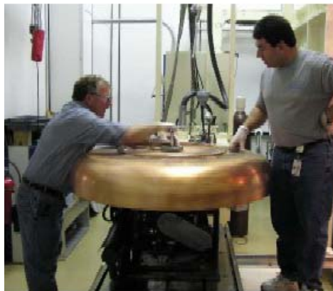
201 MHz half-shell ebeam welding of Stiffening – JLab
