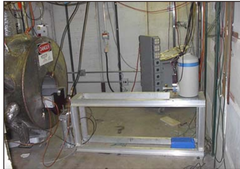
Studied dark current & X-rays from cavity with various detectors
