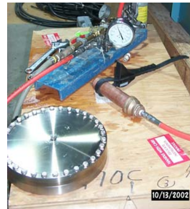
High pressure seal test for high-pressure RF studies – Muons Inc
