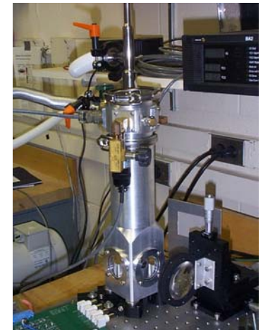
Bolometer detectors for Window Beam profile – cryogenic setup– U. Chicago
