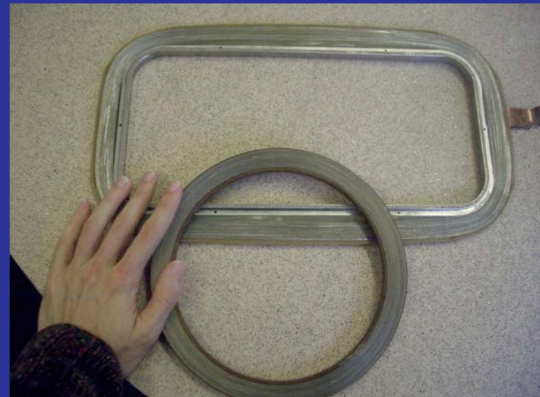
Example of BSCCO-2212 coils (Cryo department, Southampton Univ, UK)
