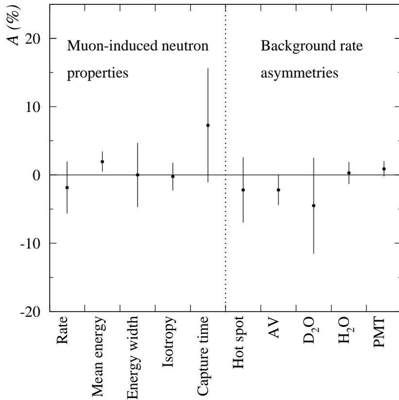
Diurnal stability of detector verified with muon-induced neutrons and radioactive background rates.
