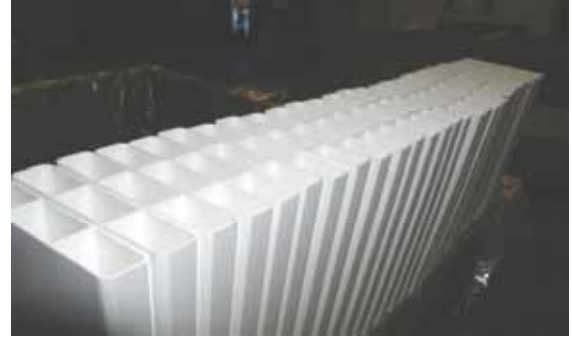
Fig. 6.6: Cell structure of the three cell prototype of extruded PVC with 12% \text{TiO}_2 .
