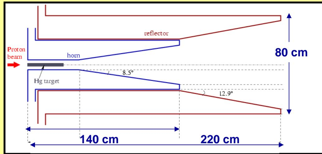
Drawing from the horn built at CERN
