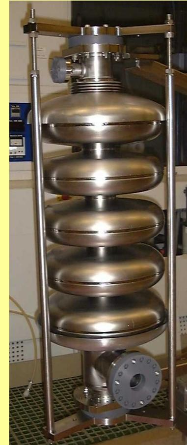
LEP cavities may have worked 350MHz & 3.6MV/m effective gradient
