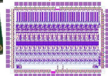
FLC_PHY3 (2004) 18ch 15 bit readout BiCMOS 0.8 \mu 2600 chips
