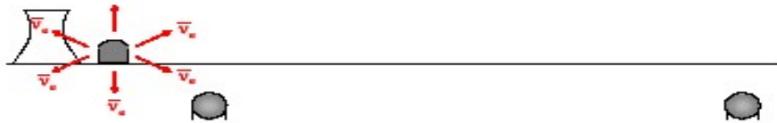
Figure 4: Schematic layout of a two detector reactor neutrino oscillation experiment.
