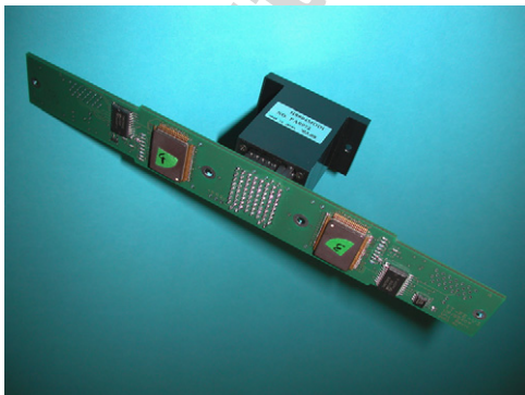
Fig. 25. The front-end PCB connected to a multi-anode PMT.
