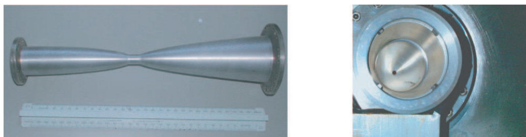
Figure 3.26: AD horn (left) and view of a broken AD horn (right) during its replacement from the beam line.
