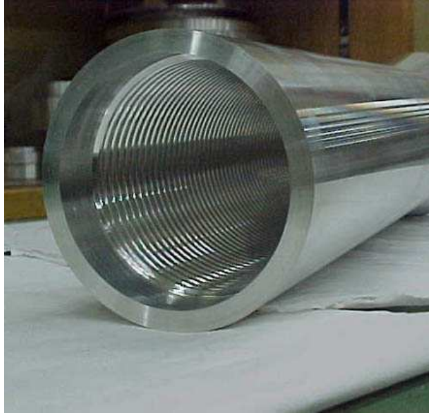
Figure 3.23: Horn neck conductor shaped like a screw to increase the thermal exchange surface.
