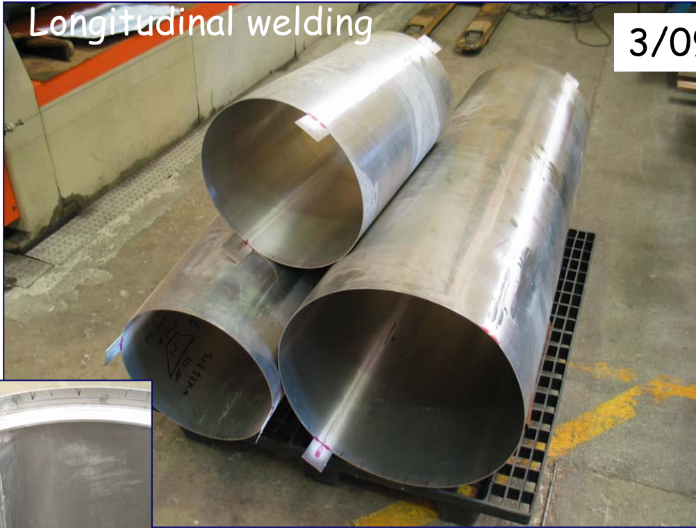
2mm Al thick plates rolled and welded
