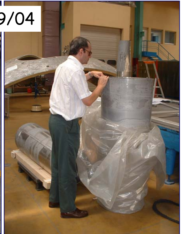
2mm Al thick plates rolled and welded
