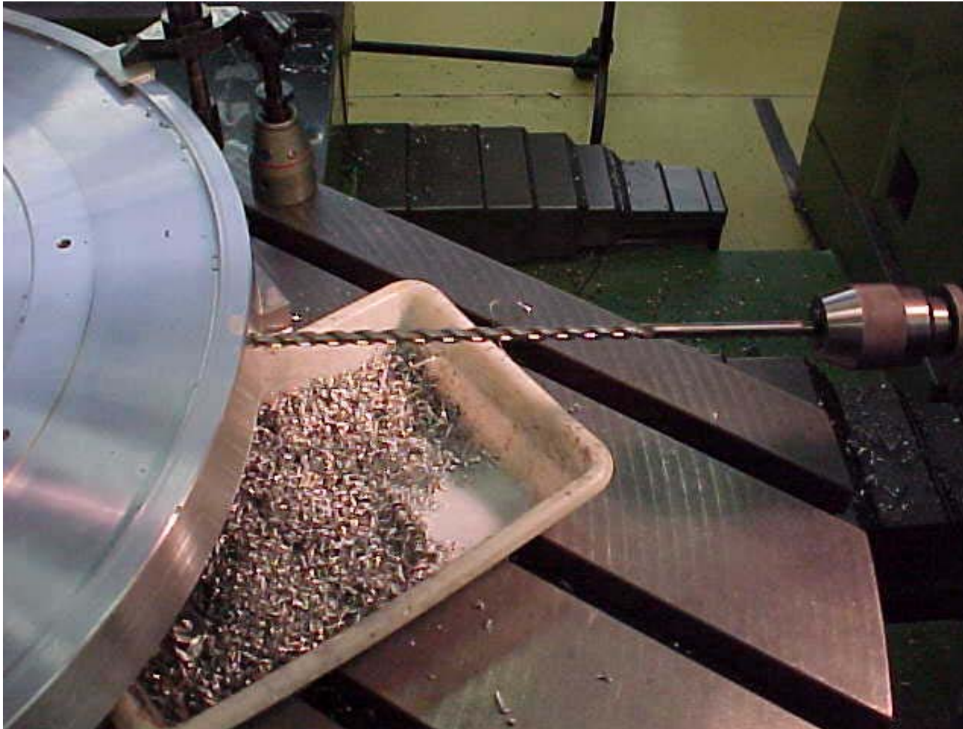
Drilling operation for radial holes
