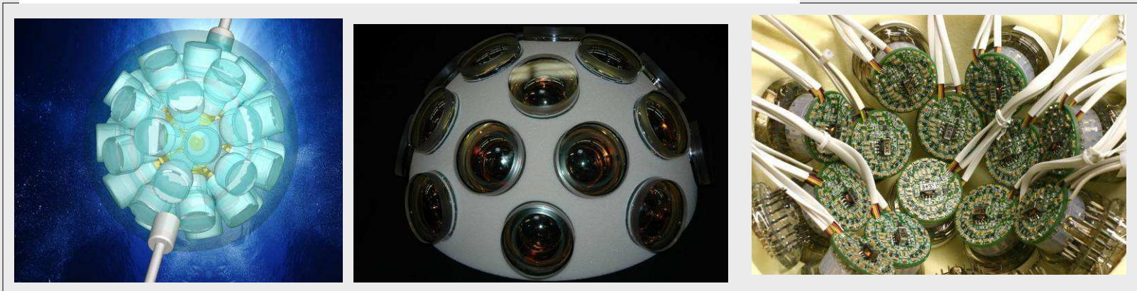
multi PMTs in one glass sphere
