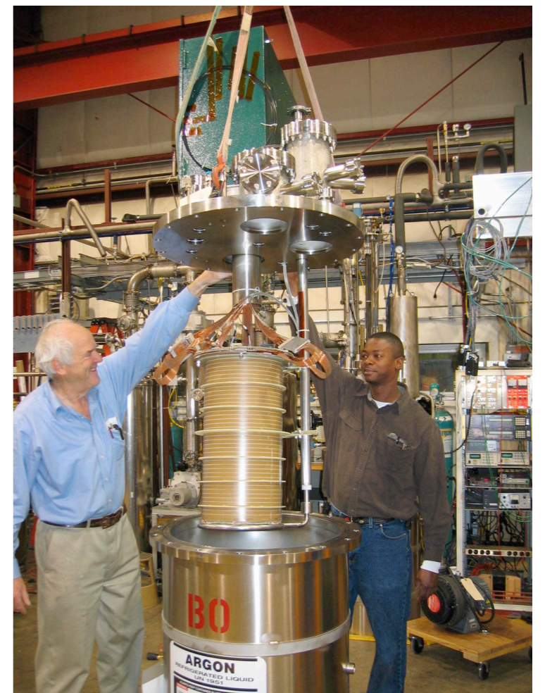
Bo TPC being installed at Fermilab
