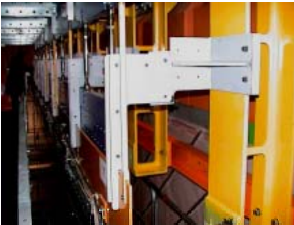
First Target Tracker flat beam alignment system
