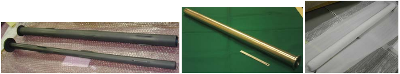
Figure 2.12: Mechanical prototypes of the target system. The left picture shows the target(bottom) and the graphite inner cooling tube(top). The center and right picture is the titanium outer cooling pipe after the welding with the downstream beam window and after the ceramic-coting, respectively.
