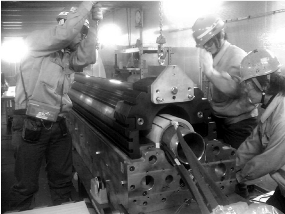
Figure 2.7: Superconducting combined function magnet assembly at Mitsubishi Electric.
