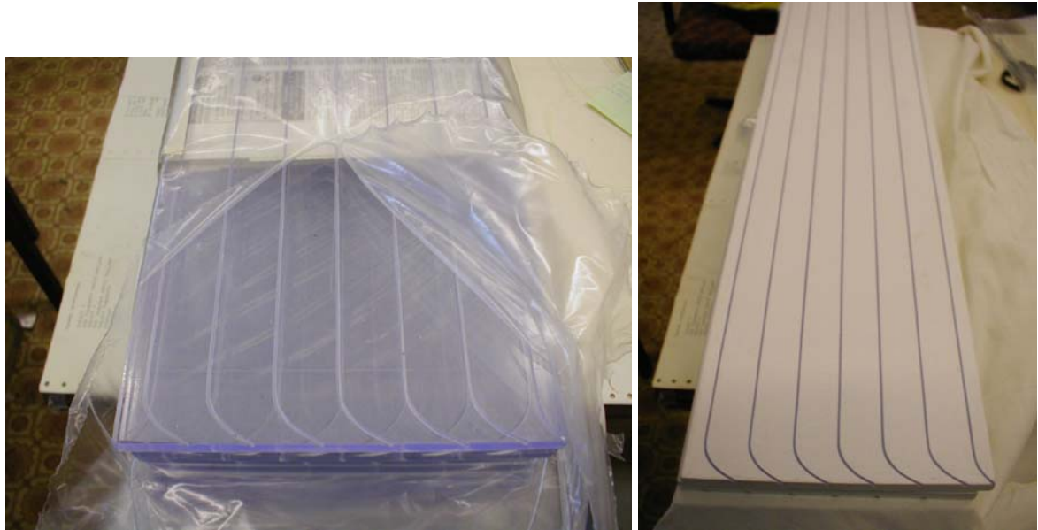
Figure 3.16: The left and right panel show a 87 cm long, 17 cm wide, and 1 cm thick scintillator with grooves to embed WLS fibers. The spacing between the grooves is 2.5 cm. The scintillator shown in the right panel is coated with a chemical reflector.
