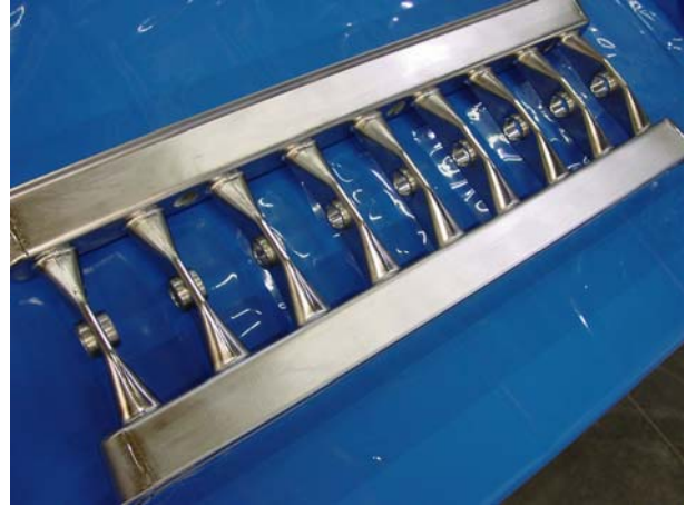
Fig. 4.3.12b: Welded Niobium girder + stem part of the sc CH-cavity for HIPPI
