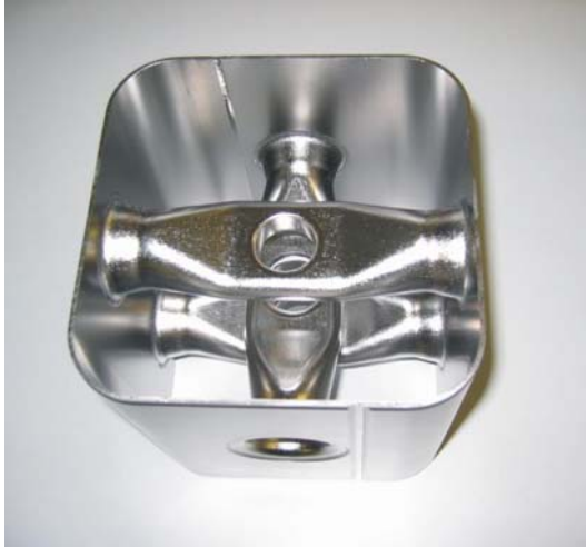
Triple spoke Nb cavity without endcaps
