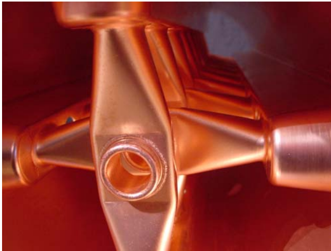
Fig. 4.3.12c: Niobium girder + stem part welded in the resonator of the sc CH-cavity
