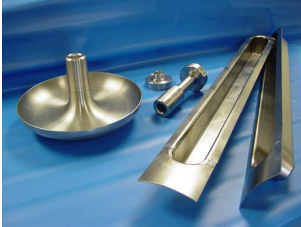
Fig. 4.3.12a: Some Niobium parts of a sc. CH-prototype for HIPPI. Tank end cell (left), two girders (right) and one drift tube part (middle)
