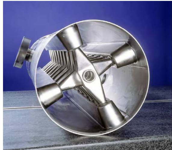
Fig. 4.3.12d: The superconducting Niobium CH-prototype cavity before the final welding of the end cells.
