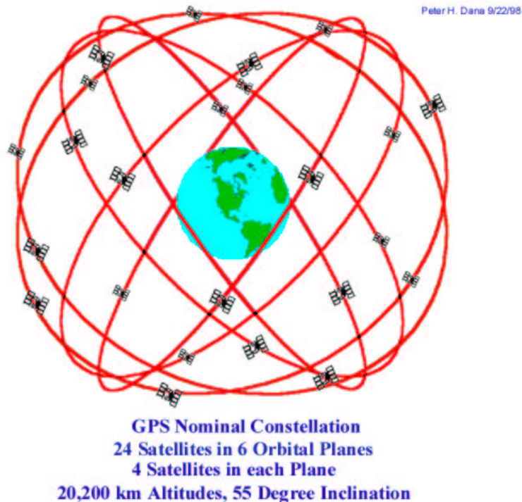
Figure 5.2: Schematic view of orbits of GPS satellites.
