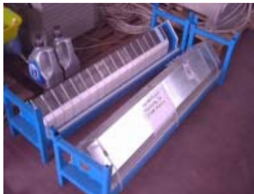
Fig. 12 Two lead transportation box with 18 plastic pallets each.
