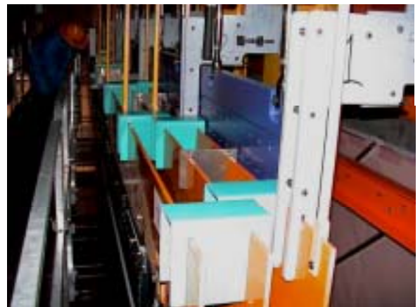
Spacers maintaining the Target Tracker flat beams straight and at the right distance between each others
