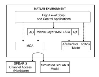
Figure 1: Middle Layer Software Flow Diagram
