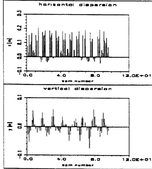
Fig.4 Measured Linear Dispersion Function
